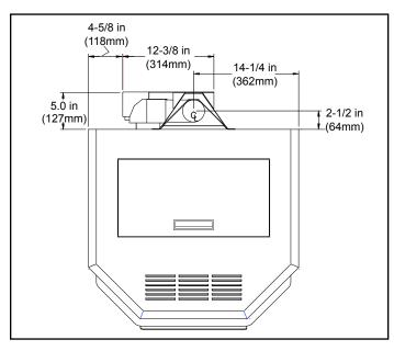
Figure 7.2 - Top View with Top Vent Adapter
